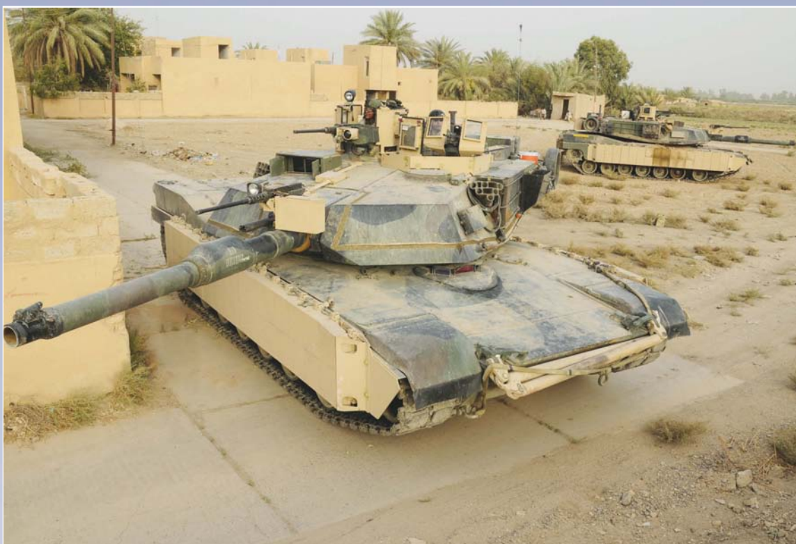
Top left: without TUSK kits the M1A1 AIM Abrams MBT has a combat weight of 61.5 tons. The vehicle is 9,827mm long (with gun forward), 2,885mm high and 3,653mm wide.
