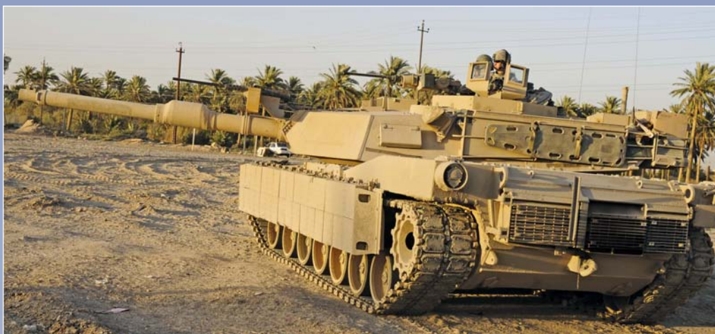
Top left: without TUSK kits the M1A1 AIM Abrams MBT has a combat weight of 61.5 tons. The vehicle is 9,827mm long (with gun forward), 2,885mm high and 3,653mm wide.
