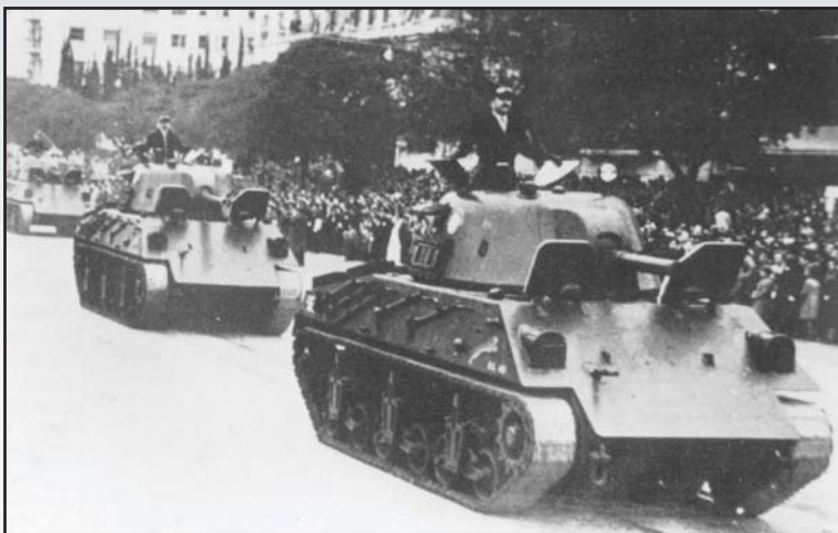
Above: DL 43 tanks seen on the military parade of the 9th July 1945 on Libertador Avenue of Buenos Aires. Two of the front machine guns were removed and they received the extra tracks on the sides of the turret. Note that the front lights are covered.
