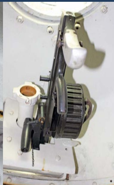
Various views showing the interior of the Renault FT17, a tank that is often seen as the 'mother of all tanks' in that it was one of the first to incorporate a rotating turret atop the hull, a design that most modern day tanks is based on. Here we see the driver's controls (top left), a view rearwards into the back of the hull (bottom left), the locking handle for the rotating turret (above left), the turret machine gun (above right), and a view looking forward from the driver's position showing the vision hatches in the closed position (right).
