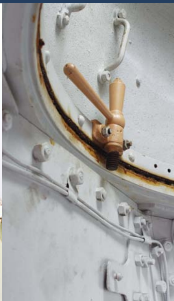
Various views showing the interior of the Renault FT17, a tank that is often seen as the 'mother of all tanks' in that it was one of the first to incorporate a rotating turret atop the hull, a design that most modern day tanks is based on. Here we see the driver's controls (top left), a view rearwards into the back of the hull (bottom left), the locking handle for the rotating turret (above left), the turret machine gun (above right), and a view looking forward from the driver's position showing the vision hatches in the closed position (right).
