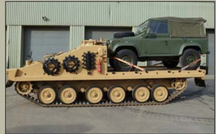
Alvis CVRT Shielder , Tracked Armoured load carrier with flat bed platform. The flat bed can adopted for a wide range of roles such as logistic carrier, bridge layer repair / recovery and towing. Built to a high specification the vehicle hull is composed of aluminium armour to protect the crew, etc. Mileage from 500, Excellent condition, Price P.O.A. (20 Available)
