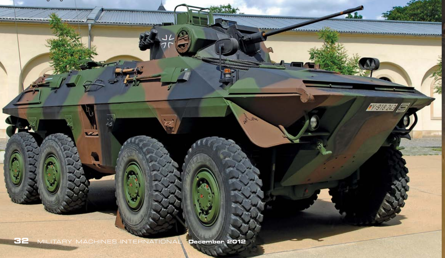
The Sp.Pz. 2-Luchs, an 8x8 amphibious reconnaissance armoured fighting vehicle that has been in service since 1975.
